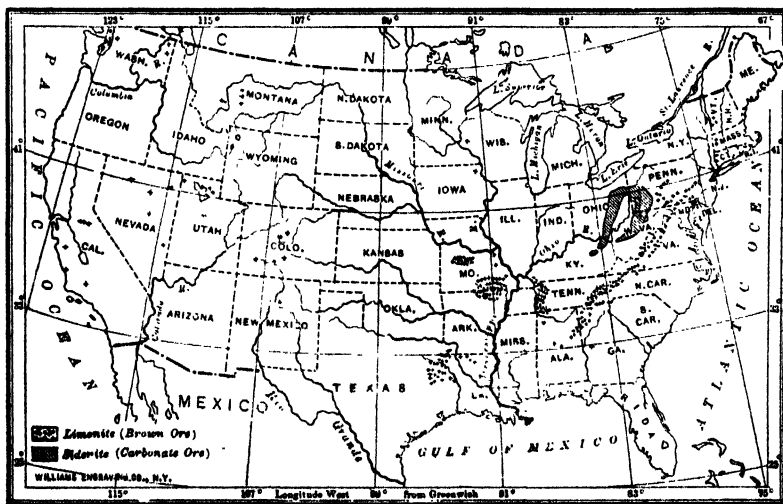
FIG. 147.—Map showing distribution of limonite and siderite in the United States. (After Harder.)
